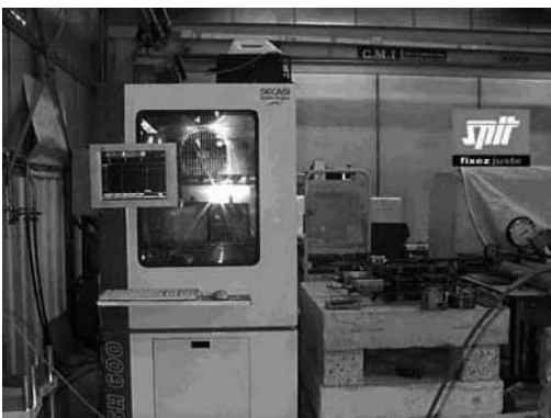
Oven to test the behaviour at high temperature chemical resins
